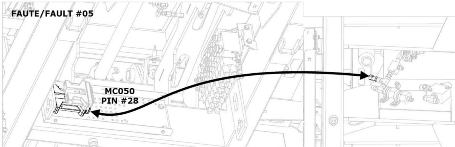
2- When this fault appears on the screen, immediately go to the touch screen diagnostic page.
